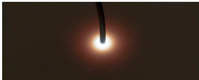
Figure 2: Photograph of the orange juice replica when illuminated by a fiber optic cable touching the top surface. The cable is connected on the other end with a white LED. We observe a color shift in the profile from white to red. We would like to emphasize that this image is a tonemapped HDR image and that the white region around the fiber optic cable is not over exposed.
