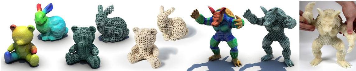
**Figure 4.17:** *The target Young's modulus distributions (colored), synthesized geometry (green) and fabricated model of the Bunny, Teddy and Armadillo.*
