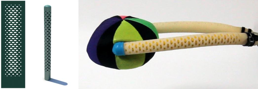
**Figure 4.16:** *The optimized structure for the gripper (left), the generated model (middle). The fabricated result (right) can be used to grab and lift small objects.*
