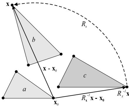
Figure 3: If the rotational part  $R_x$  of the deformation  $\mathbf{x}$  is known, the forces can be computed with respect to a deformation  $R_x^{-1}\mathbf{x}$  that only contains translation and stretching. Here, the original element (a) is deformed (b), and then rotated back into the original coordinate frame (c).
