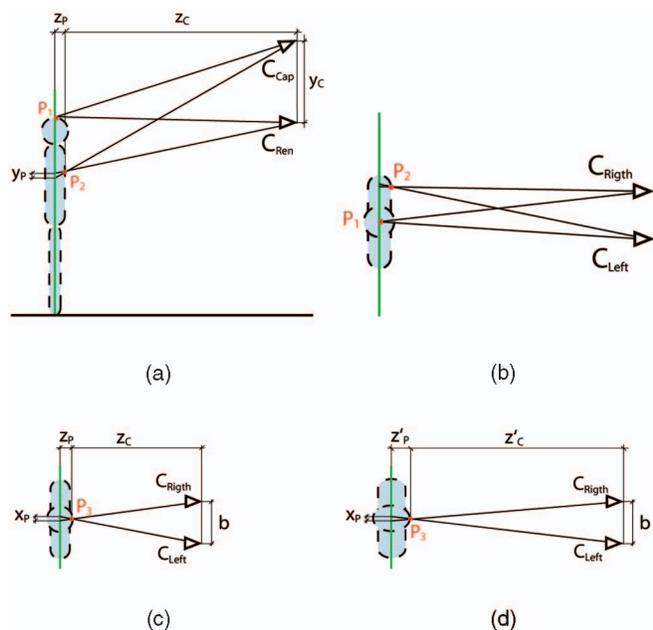
Fig. 13. Different drafts of the setup configuration are depicted (a) from the side and (b) from the top considering reprojection onto the green billboard. In (c) and (d), a rendering setup for two different viewing positions are shown.
