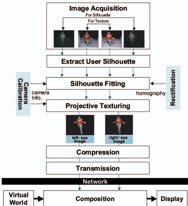
Fig. 2. System overview: the processing pipeline for the creation of stereo video avatars based on IR segmentation.
