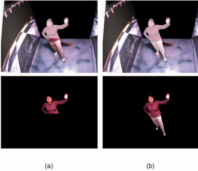
Fig. 4. Influence of IR back lighting versus front lighting. (a) Simulated mask and segmented image when using IR back lighting techniques. (b) Generated mask and segmented image when using IR front lighting techniques.
