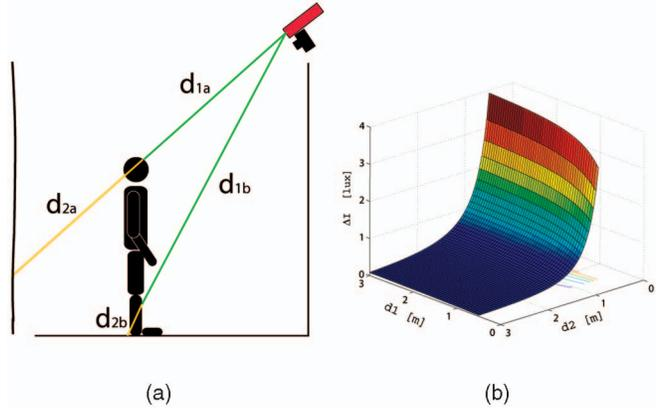
Fig. 6. Intensity depending on distance from IR light source to object. (a) Illustration of possible distances. (b) Graph showing intensity difference depending on  $d_1$  and  $d_2$ .
