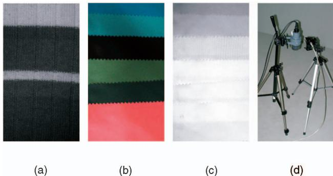
Fig. 7. IR reflection properties of different materials. (a) Part of a sweater consisting of one single material, but colored with different dyes. (b) Texture image of different color patches of the same material (c) and their IR reflection. (d) System used to scan material.
