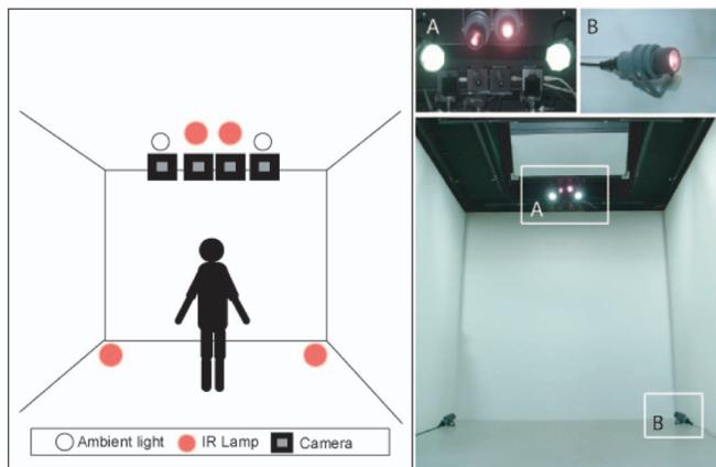
Fig. 3. Sketched and photographic view of the hardware setup, showing four IR lamps, four cameras, and two ambient lights. (a) Scaled view of one of the four used IR lights. (b) Scaled view of the specific arrangements of the components.
