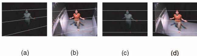
Fig. 10. Epipolar lines for color and texture images (a) and (b) before rectification and (c) and (d) after rectification.
