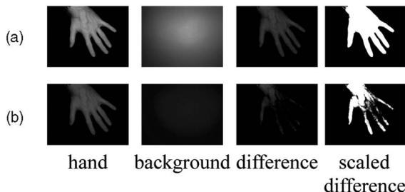
Fig. 8. Segmentation of skin. (a) Hand and Background are at the same distance from the IR light source. (b) Hand is at 1 meter and Background at 1.8 meter from the IR light source.
