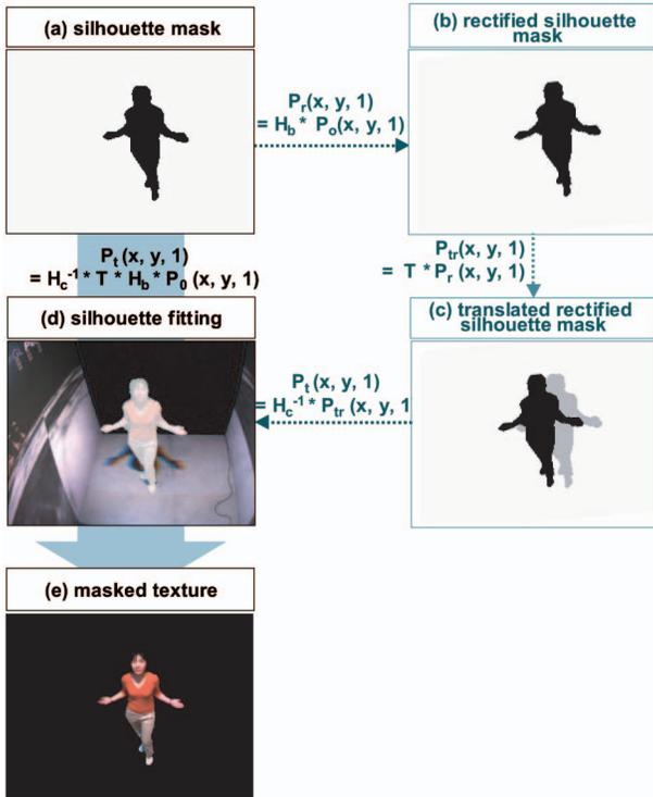
Fig. 11. Silhouette fitting process:  $P_o(x, y, 1)$  is a pixel position in the silhouette mask,  $P_c(x, y, 1)$  is a pixel position in texture image,  $H_c$ ,  $H_b$  is a homography for the rectification of the texture and silhouette image, respectively.
