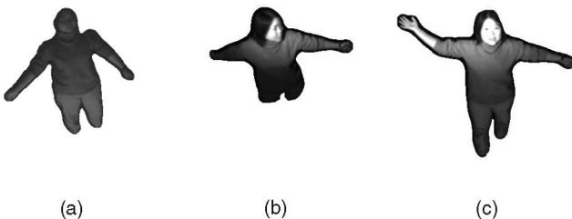
Fig. 5. Segmentation depending on different setups of the IR lights. (a) IR lights only on the floor. (b) IR lights only on top of the front wall. (c) Combination of the two previous setups.
