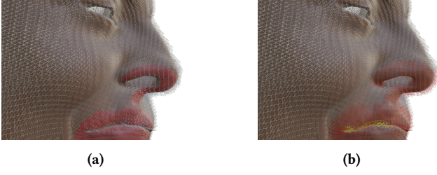
Figure 2: (a) We use the underlying embedded surface mesh of the face as the proxy for collision response. Specifically, the collision proxy is mainly the mouth region (red). (b) The simulation mesh could be divided into the collision-agnostic part (gray, n_1 vertices) and the collision-aware part (red, n_2 vertices) that embeds the proxy. During simulation, only a small fraction of the proxy vertices are activated in the constraint set C and affects the simulation mesh (yellow, n_c vertices). Note how the magnitude of these three hierarchies differ.
