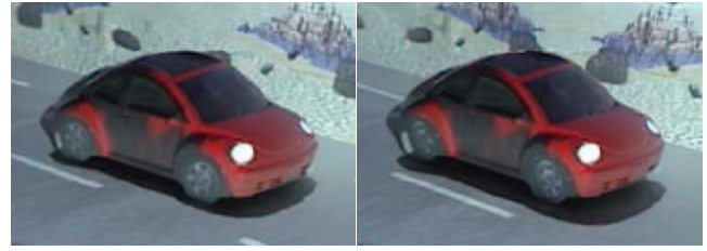
Figure 3: Vertical displacement by shifting the background and shadows. These two pictures are taken from the same camera position, so the car in both images is at the same location. Note (i) the change in position of the virtual shadows and (ii) the parallax for the edge between ground and backdrop with respect to the right headlight.
