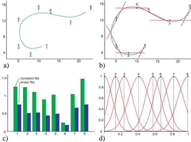
**Figure 7:** Curve reconstruction: a) Reconstruction with constant fitting functions. b) Reconstruction with linear fitting functions. c) Absolute error at the data points. d) The reconstruction functions in the parameter domain.
