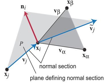
**Figure 4:** Computing directional derivatives using normal sections. patch, hence we ignore it. This procedure is sufficient to handle patches with boundaries. Next, we compute the direction  $\tilde{\mathbf{v}}_j$  of the intersection line of the plane  $P$  and the plane given by  $\mathbf{x}_i$ ,  $\mathbf{x}_\alpha$ , and  $\mathbf{x}_\beta$  (see Figure 4).
