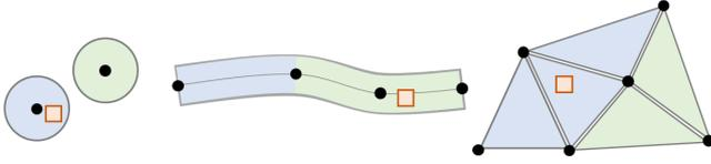
**Figure 3:** Terminology used for points, lines and surfaces: vertices (black points), segments (green and blue), fragments (orange).
