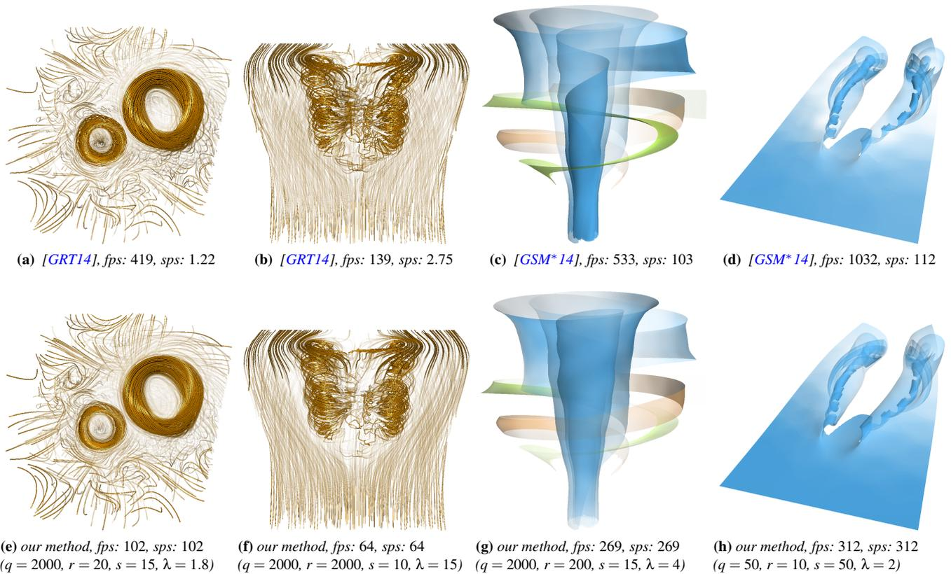
**Figure 12:** Comparison of [GRT14] and [GSM\*14] (top row) with our decoupled opacity optimization (lower row). The results are visually similar. The solves per second (sps) increased significantly, whereas the frames per second (fps) reduced, since our opacity computation runs on the GPU, not the CPU. While previous method solved for the opacities asynchronously, our method can calculate it every frame.
