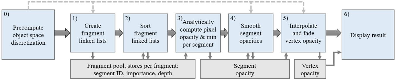
**Figure 2:** Overview of the rendering pipeline, see Section 4.1 for details. Blue boxes denote the subsequent rendering stages and gray boxes represent memory. The dashed gray lines indicate stages that use the precomputed object-space discretization.
