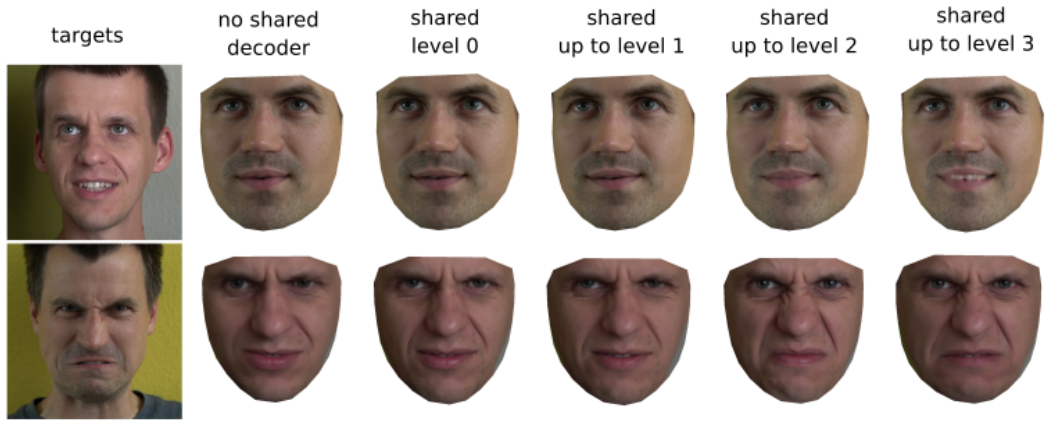
Figure 12: Output of the network with various number of shared decoder levels. The target image is presented on the left side. Images from left to right correspond to the output of the network with the split placed after: latent vector, level 0, level 1, level 2 (which is our choice) and level 3.
