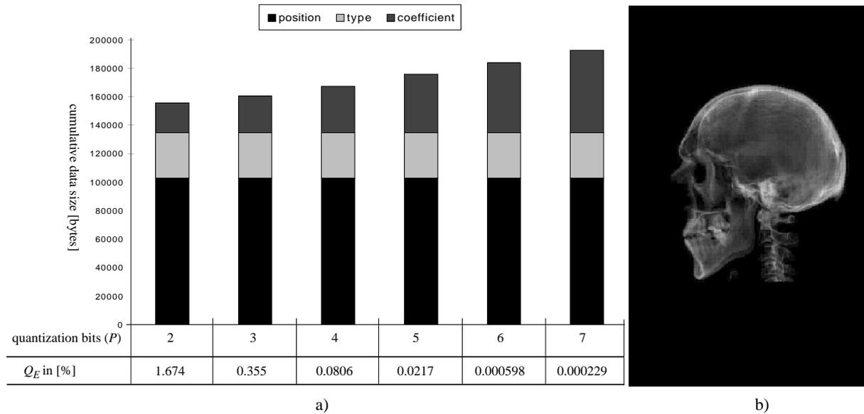
**Figure 16:** Relation between data size and number of bits for quantization (data source: Visible Human Project, CT-data set). Volume size:  $256^3$ , max. decomposition level  $M=3$ , no. of splats 74340. a) proportions of coefficient, type and positional data and resulting data size.. b) reference image of compressed data set.
