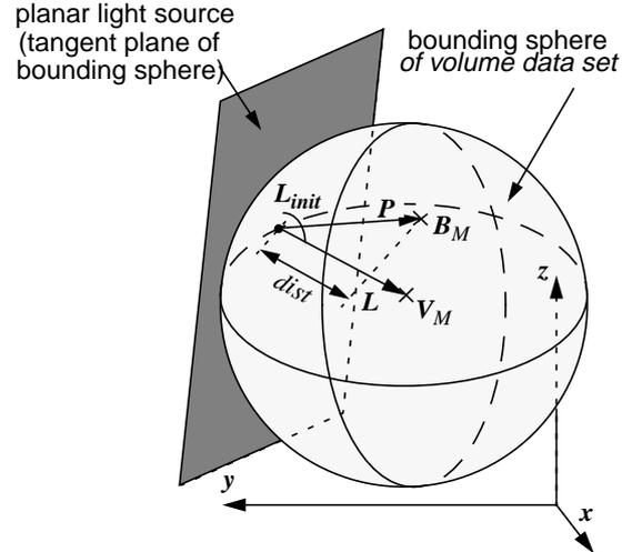
**Figure 7:** Geometric relationships for distance-weighting of basis functions.
