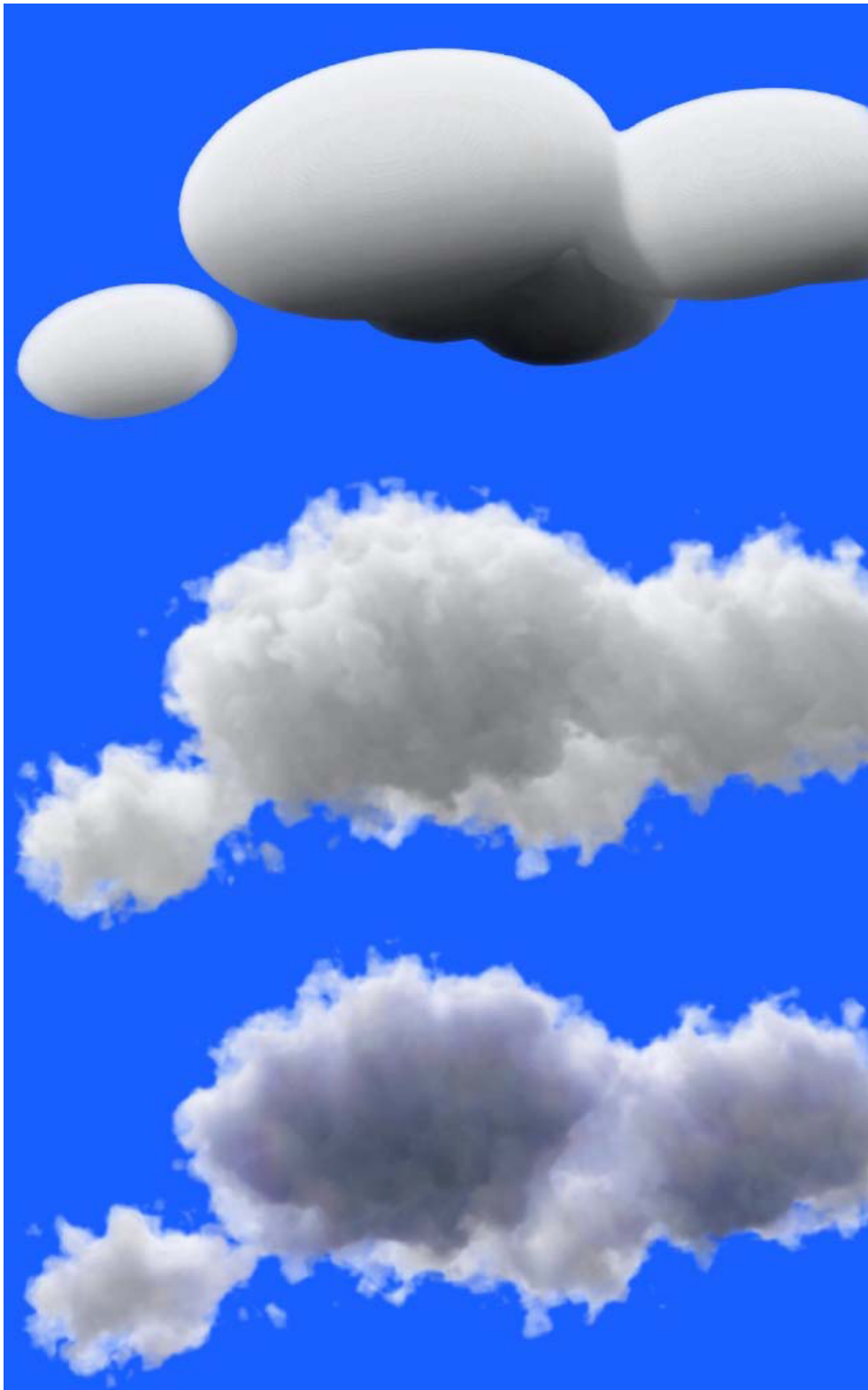
Figure 49.1: Procedural clouds. The image on the top shows the underlying data, 64^3 . The center image shows the perturbed volume. The bottom image shows the perturbed volume lit from behind with low frequency noise added to the indirect attenuation to achieve subtle iridescence effects.
