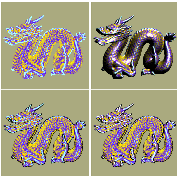
Figure 33.5: Dragon distance field (128x128x128) with colors from curvature magnitude (top, left); with Phong shading (top, right); with contours (bottom, left); with ridge and valley lines (bottom, right).
