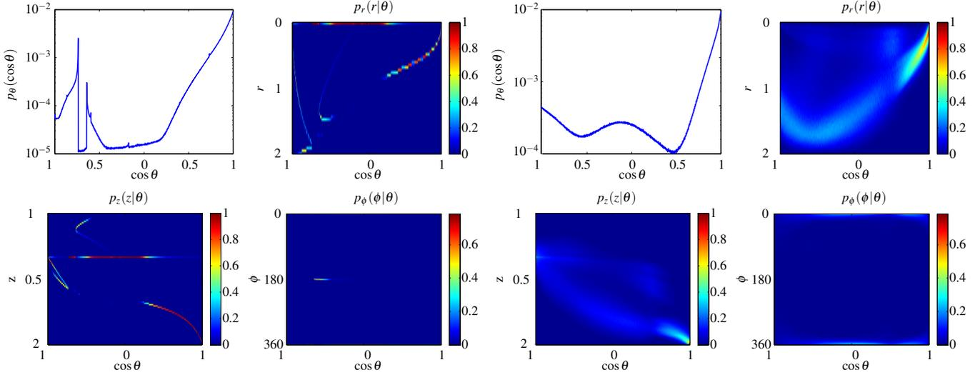
**Figure 1:** The TSDF of a dielectric sphere with index of refraction  $\eta = 1.33$  (left two columns) and our snow grain (right two columns). The arc-like structures in the plots are due to internal reflections. Note that the graph for  $p_\theta(\cos \theta)$  for the dielectric sphere has been validated against literature (cp. [Zhou et al. 2003, Fig. 8]).
