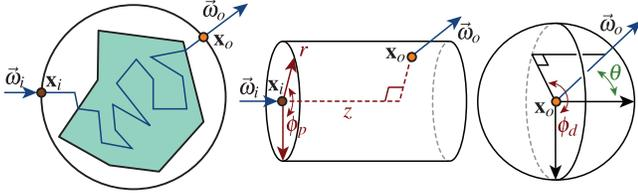
**Figure 2:** Our notation as well as the cylindrical and spherical coordinate systems used for TPT.
